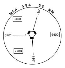
But suppose you are being vectored below the MSA? This is an approved procedure used by ATC to facilitate traffic sequencing. The Minimum Vectoring Altitude (MVA) chart (known only to radar controllers) shows obstructions on the radar screen template. This allows more
